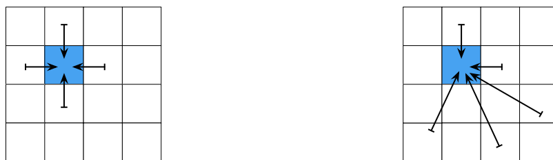
(A) Communication pattern in a regular application. (B) Communication pattern in a graph application.
